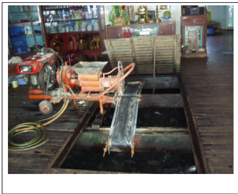
Figure 3: A food grinding machine on a raft, on which people live together with the catfish
